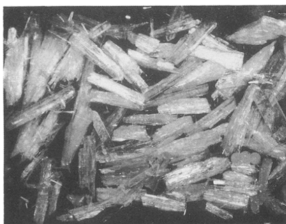
Figure 8 Collection of fibres detached from a fibrous spherulite showing single crystallinity of the fibres. ( \times 25 )
